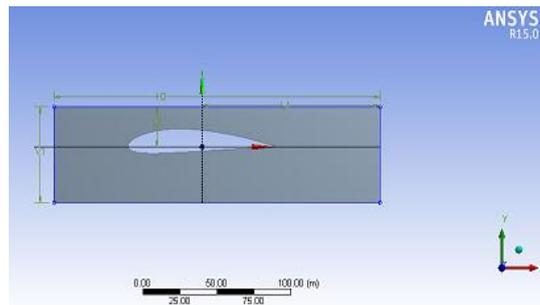
**Figure 2: Geometry of NACA 4415 Aerofoil**
