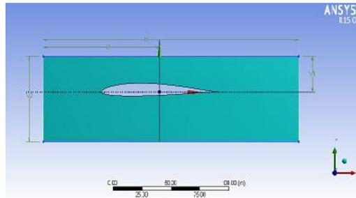
**Figure 1: Geometry of S6061 Aerofoil**
