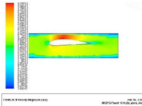
**Figure 10: Contour of Velocity Magnitude of NACA 4415**
