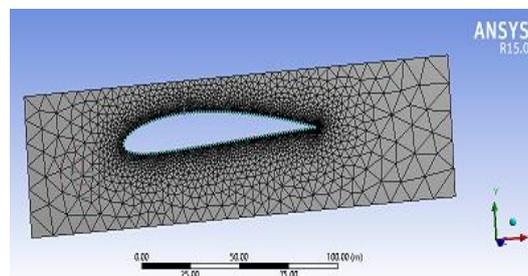
**Figure 4: Meshing of NACA 4415**
