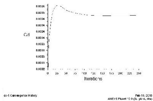
**Figure 16: Convergence Plot of  $C_D$  of NACA 4415**
