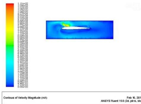
**Figure 9: Contour of Velocity Magnitude of S6061**
